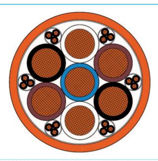
Application: For the application as fixed supply cable easy to install or for flexible use without elevated mechanical stress for hand-held applications for example mobile GPUs. Optimised flexibility due to smooth core and sheath materials that allows easy installation and handling.
